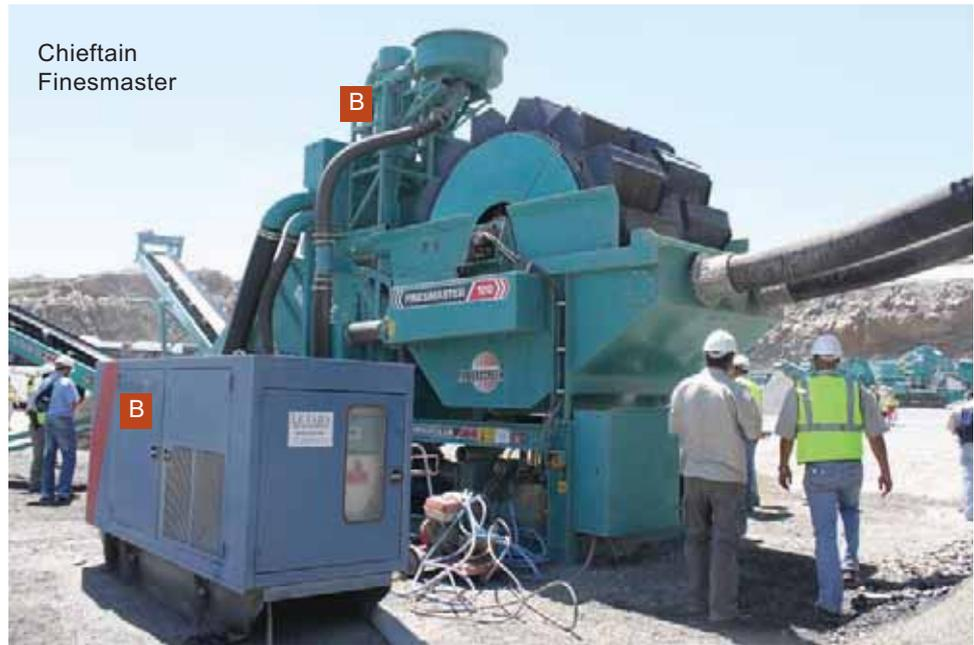
The plant washed 11 - 15 mm, 8-11 mm and 6 - 8 mm sand, as well as 0 - 6 mm concrete sand.
