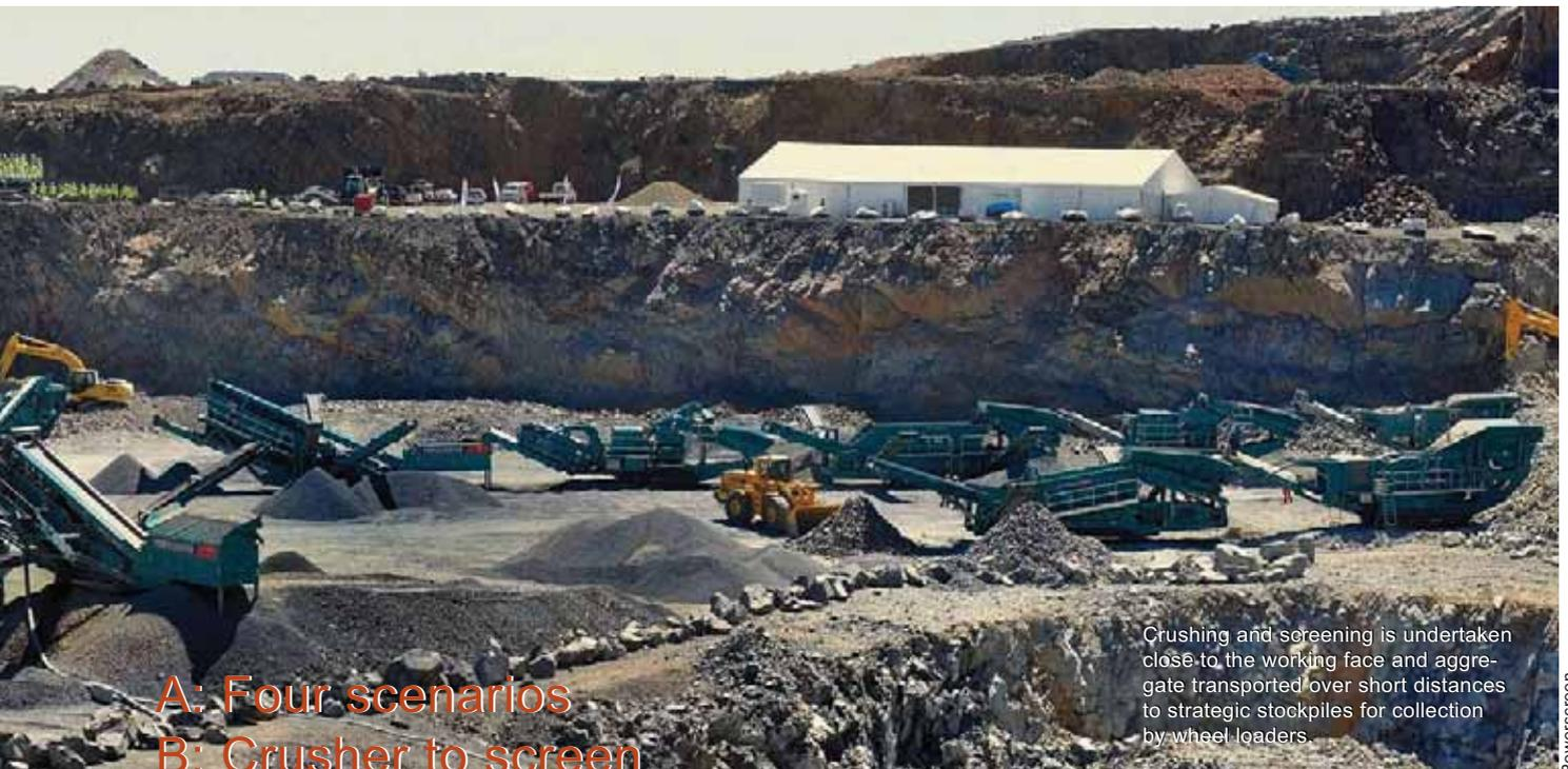
Crushing and screening is undertaken close to the working face and aggregate transported over short distances to strategic stockpiles for collection by wheel loaders.
