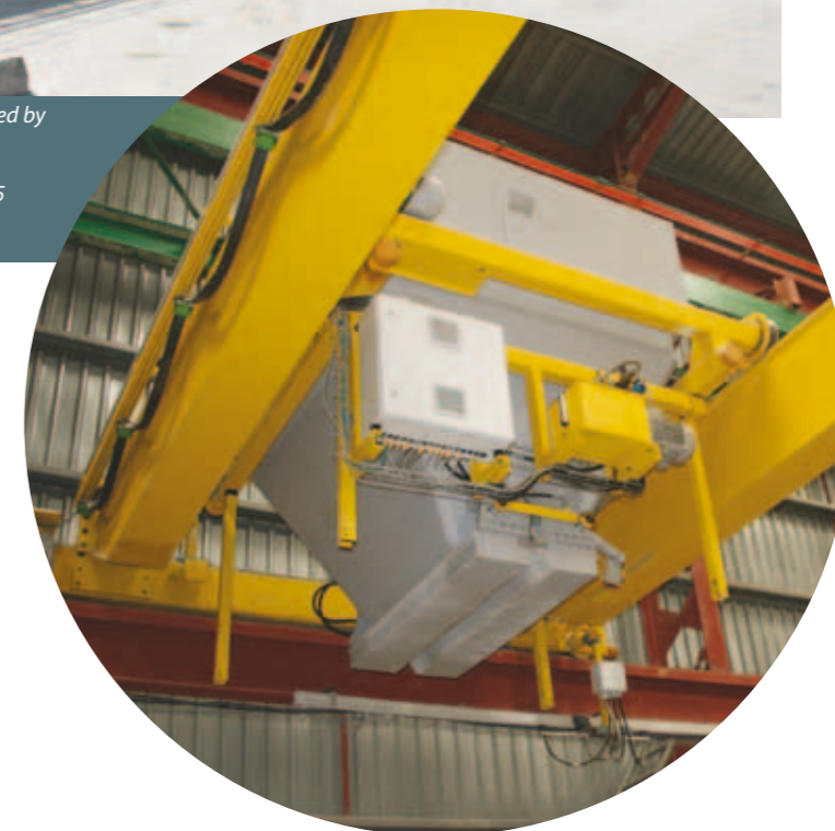
Right: The concrete is carried directly from the mixing plant by the EB405 aerial shuttle which places the material directly over the bucket gantry, discharging the batch into the extruder.
